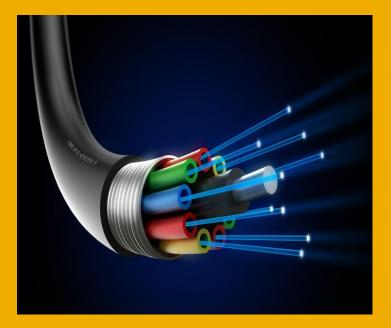
A glass or plastic strand that transmits information using light and is made up of one or more optical fibres enclosed together in a sheath or jacket.
